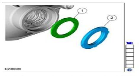
Clean and inspect the transmission case and bearings. Check for leaks from plugs and park pawl actuator rod sleeve. Repair or replace as necessary.
