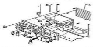
The SCR panel has a thermal conducting material applied to its undersurface and care should be used when handling control to avoid contaminating other items when storing panel.
