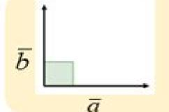
$\overline{a} \bullet \overline{b}$  are orthogonal (perpendicular) if and only if  $\overline{a} \bullet \overline{b} = 0$
